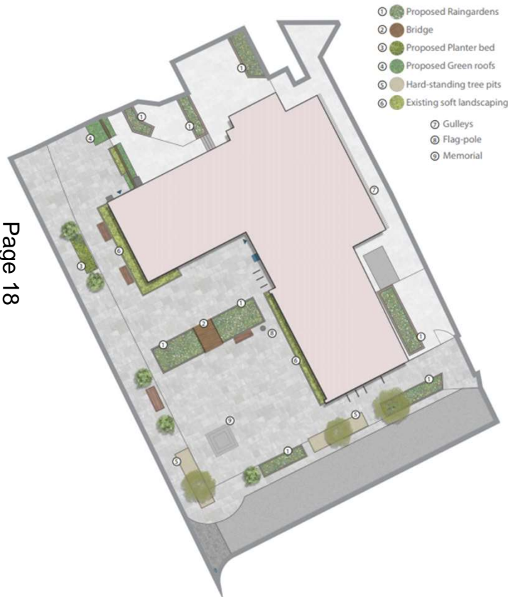
① Rain gardens - SuDS that capture rainfall before it enters the piped network and allows it to infiltrate into the ground.
